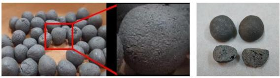
Fig. 5 – Particle shape, color, and surface texture of  $(A_{GP})$
